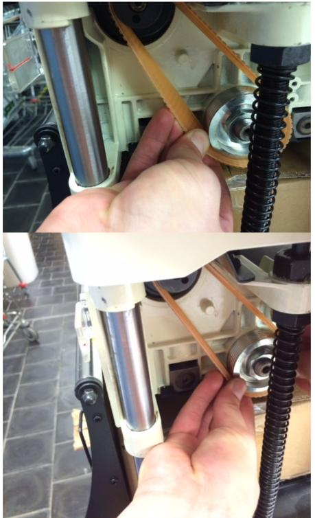
Tilt the belt and during rotation move the belt in other one or two teeth towards . Repeat this procedure until the belt will be in right position see next picture.
