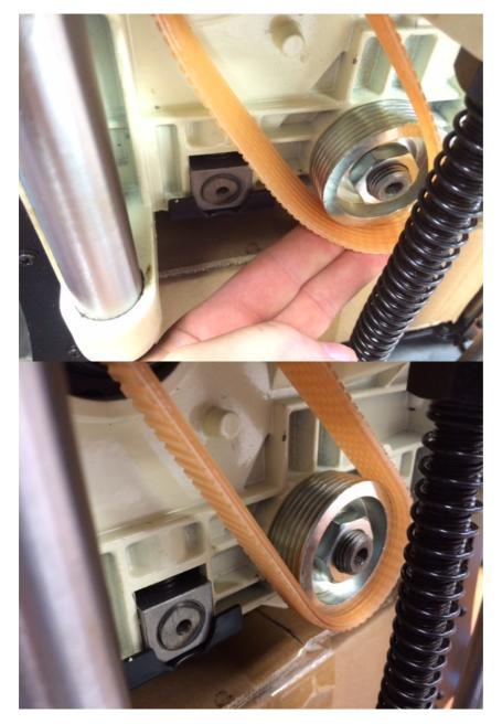
Then put driving belt on the bottom silver wheel at first one or two teeth . Rotate with wheel in order to belt put on the wheel .
