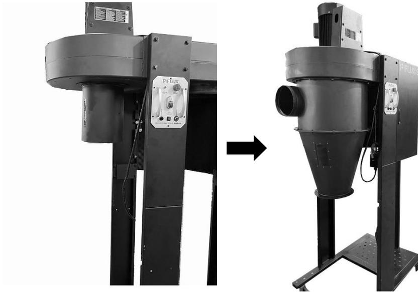
Step 10: Secure the filter cover using (4x) 1/4"x3/4" bolts and (4x) 1/4" washers.
