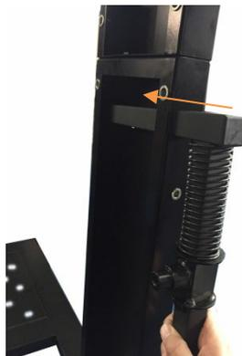
Step 26: Make sure the bar is pushed all the way into the opening on the lower upright support. Secure the bar using (4x) 5/16"x1-3/4" bolts, (8x) 5/16" washers and (4x) 5/16" nuts. Follow the same steps for the opposite side.
