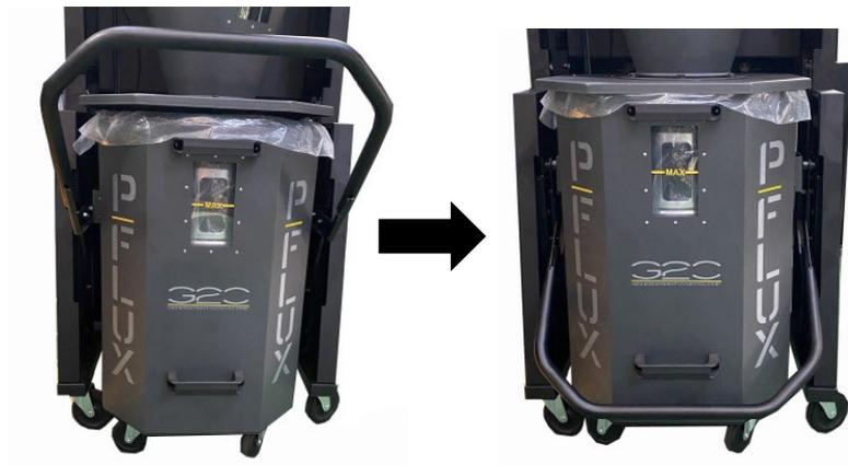
Step 47: Make sure when aligning the drum that both the left and right side plates are seated in the lifting mechanism (A). When aligned incorrectly (B), the drum will not be fully sealed and will interfere with the airflow.
