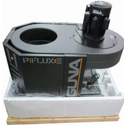
Step 2: Remove base frame that is bolted to (3x) top upright supports. Keep (6x) 3/8"x3/4" bolts and (6x) 3/8" washers.
