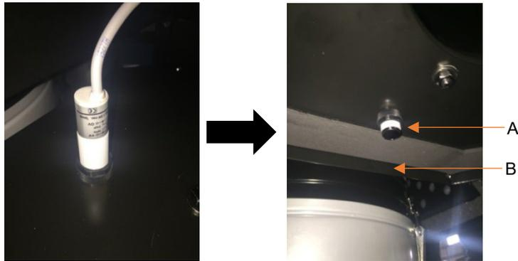
Step 34: Attach the LED light to the drum lid using (6x) M4\*10mm bolts, (6x) 3/16" washers and (6x) M4 nuts.
