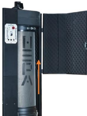
Step 21: Attach the filter end cap to the HEPA filter using the (4x) latches. Cover the opening with a rubber plug.
