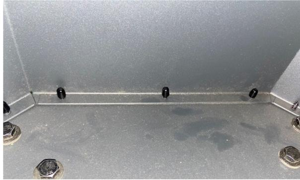
Step 42: Once assembly is complete, apply silicone (not included) to the top and bottom rim inside the drum. This will seal the drum and prevent any leaks.
