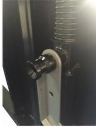
Step 31: Secure the bar to the handle using (2x) 3/8"x21mm bolts and 3/8" nuts. Make sure the bolt head is on the inside of the handle (A). Adjust the tightness of this bolt accordingly. If this bolt is too tight, the lifting mechanism will not work smoothly. When too loose it will not pick up the drum.
